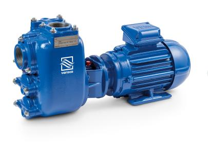
**Product Data** Suction port Threaded - 2" ISO 228 (BSP) Delivery port Threaded - 2" ISO 228 (BSP) Qmax 44 m<sup>3</sup>/h - 733 l/min (193 USgpm) Hmax 20 m (65 ft) Solids handling 25 mm (1") Motor power 2.2 kW - 3 HP Motor type **IEC** standard Winding for inverters **Cast iron frame** Motor brand WEG W22 Premium Weight 60 kg (132 lb)
